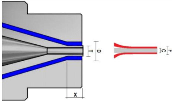
The head should allow the fine centering if fine concentricity adjustment is required.
