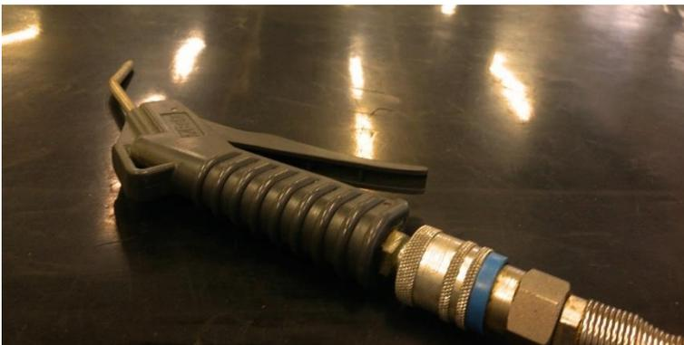
Figure 4 - Compressed air gun
